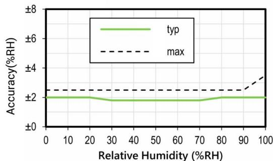
4. Typical RH accuracy corresponding to the temperature.
